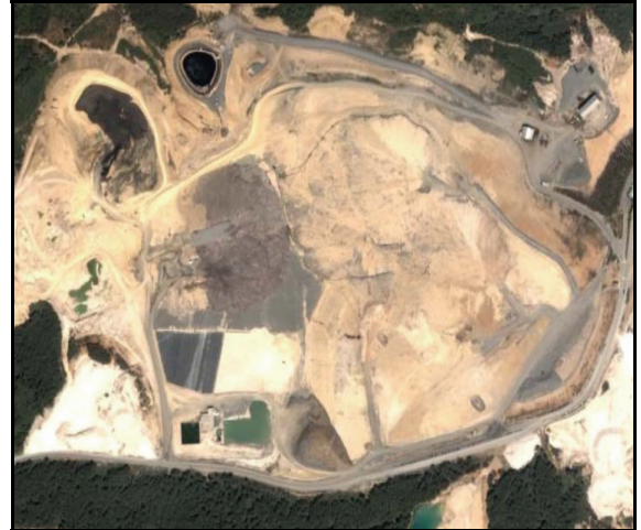
Figure 5. An aerial view of the Komurcuoda site. Maximum depth of waste is 70 m, average 19 m.
